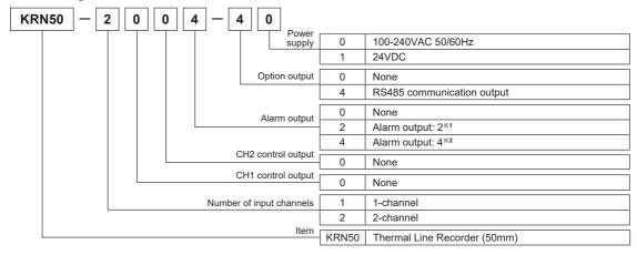
X 1. When selecting this for 2 CH model, two alarm outputs for CH1 are available. In other words, you cannot set one for CH1 and one for CH2.
