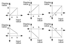
Display scale function is able to change display value for max./min. measured input by setting high limit scale [ Hi Scale ] and low limit scale [ Lo Scale ].
