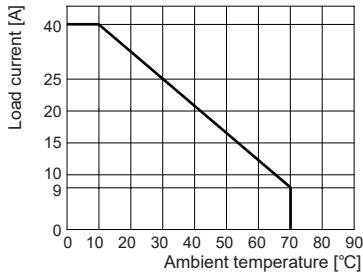
⚠ Since effectiveness of the heat radiation is decreased when multiple SSRs are installed closely, please supply less than 50% of the rated load current.
