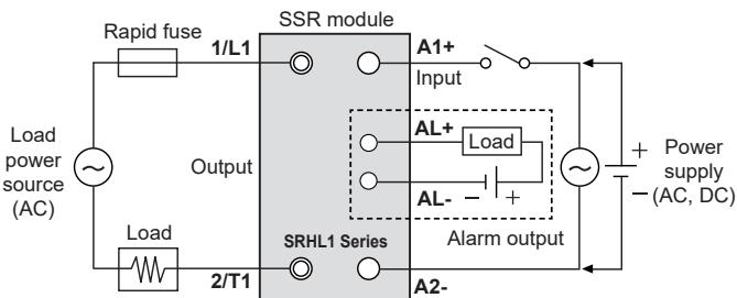
※Alarm output terminals (---) are only for the rated load current 40A model (SRHL1-□□40□).
