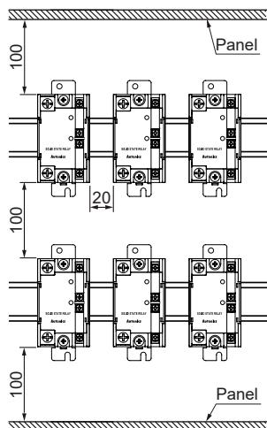
※ When installing multiple SSRs, please keep space between SSRs for heat radiation. When installing SSRs horizontally (input part and output part on the same height), please supply less than 50% of the rated load current.
